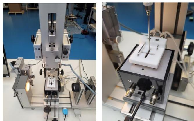
Fig2: TRACKER™ equipped with the Dense phase exchange module
